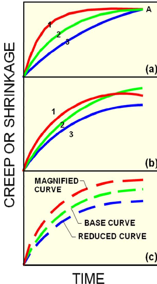
FIGURE 3-1 OPTIONS FOR TREATMENT OF CREEP AND SHRINKAGE WITH TIME
